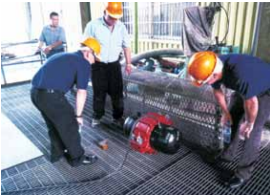
Proof and burst pressure testing
