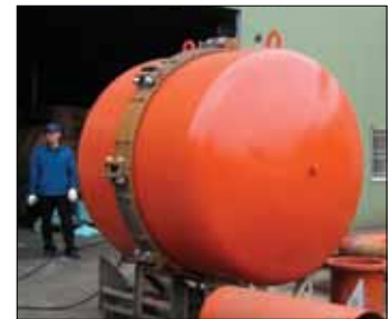
Hydrostatic testing - 72' R-88 coupling
